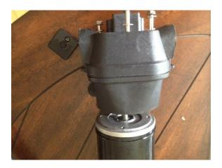
Note that the pump head starts from the stainless-steel ring as per picture.
